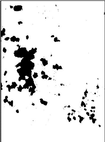
Rust Grade 4-G, 10% Rusted
