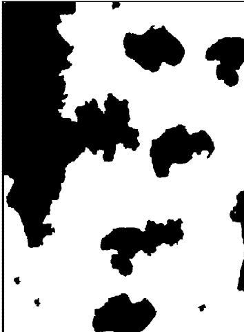
Rust Grade 2-G, 33% Rusted
